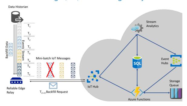
This sample implements a new communication protocol to enable reliable upstream communication from IoT devices. It automates data gap detection and backfill.
