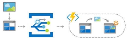
Event Grid can trigger Azure Functions, Logic Apps, or your own custom code. A major benefit of using Event Grid is that it uses a *push* mechanism to send messages when events occur. The push architecture consumes fewer resources and scales better than *polling* mechanisms. Polling must check for updates on a regular interval.
