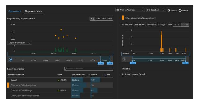
The custom telemetry reveals the average time to insert a new row is 32.6 milliseconds.
