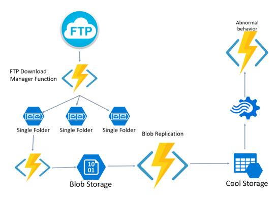
In the diagram, "cool storage" provides data that is parsed in <u>Azure Stream Analytics</u>. Any issues encountered in the data stream trigger an Azure Function to address the anomaly.
